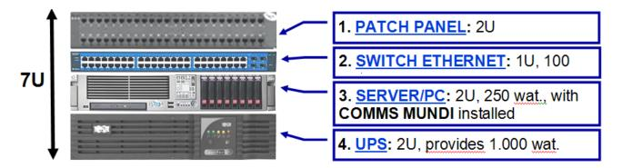
panel, a small switch and a server in which it is installed.**COMMSMundi**. The space required would be around 7U, a small fraction of what a standard installation occupies. However, this solution could serve networks of several thousand users with the use of a powerful server. This reduced space allows installation in virtually any location, a great advantage over the traditional alternative.
